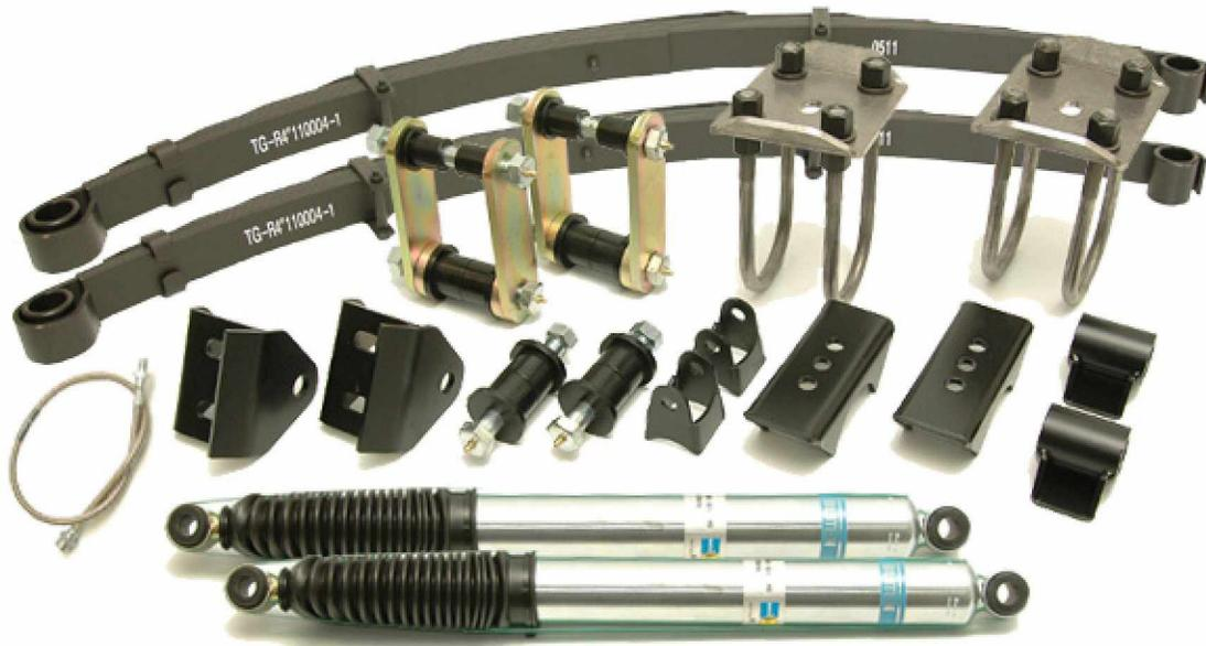
Trail-Gear Rear leaf springs are longer than stock springs and require the spring hangers to be relocated further apart. To begin installation, raise truck using large secure jack stands. Remove rear axle, drive shaft, shocks shackles, and leaf springs.
