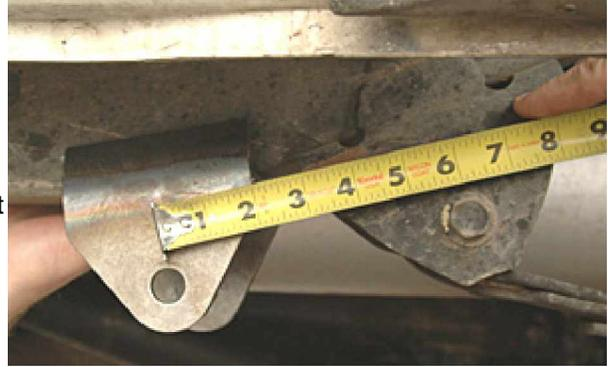
For 1989-1995 Pickups only. The 1989-1995 Pickups used longer spring than the earlier trucks. Follow the spring hanger mounting instructions above but change the dimensions from 6" to 5" so that the hanger is mounted 5" forward of the stock mount.
