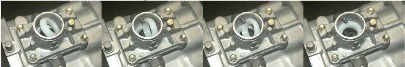
13. Install the shifter extension onto the transmission shifter. The transmission shifter will use the extension with the ball end. It will also use the two keepers to position and retain the extension onto the shifter.
