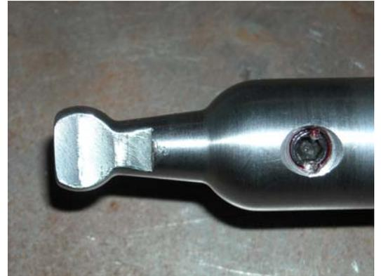
**ATTENTION: After installing the short shifter there should be no excessive play or travel in the shifters. If, after time, you notice more play in the shifter, remove the shift tower and inspect the shift extensions to verify that the set screws have not come loose. If the set screws come loose they can fall into the transmission and cause transmission failure.**
